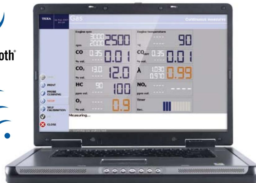
The Wireless *Bluetooth* connection allows GASBOX Autopower and RC3, its RPM detecting interface, to communicate with the display (any PC, ECO PEGASO fixed station, or AXONE Palm or Pad) without wires.
